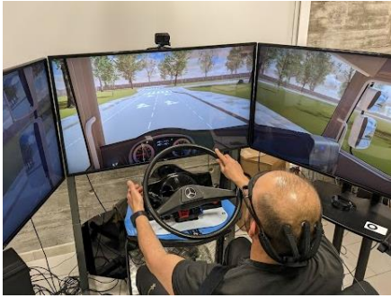
Figure 1. Picture of the experimental setup, with the driver seat in the simulator and wearing measurements devices.
